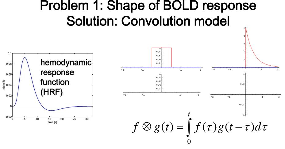
The response of a linear time-invariant (LTI) system is the convolution of the input with the system's response to an impulse (delta function).
