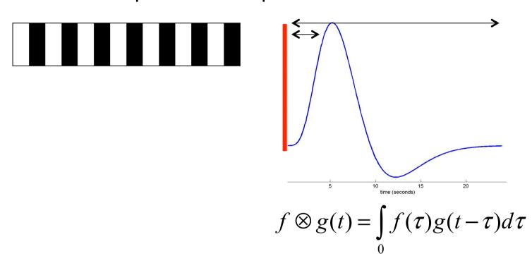
The response of a linear time-invariant (LTI) system is the convolution of the input with the system's response to an impulse (delta function).
